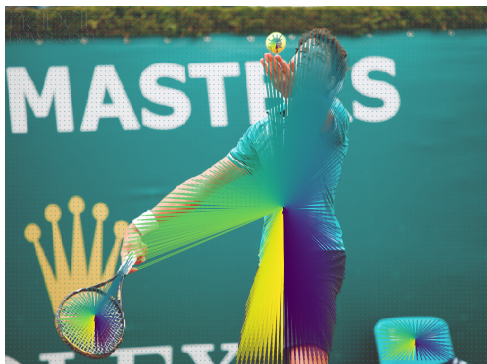
Figure 3: Center of mass regression map. Foreground pixels of masks are activated to regress the center of mass of the object they belong to. Colors are encoding the angle of the vector for a better visualization.
