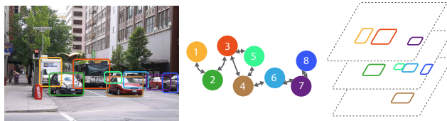
Figure 4: Graph coloring problem. Given a set of overlapping objects, find the minimal set of masks without bounding box overlaps.
