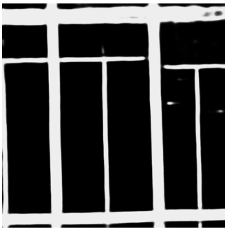
Figure 2. A prediction from our encoder-decoder CNN model. We can observe the presence of holes in the top-right road.
